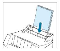
The automatic input tray holds 150 sheets of paper and five sheets of special media. See "Media Sizes and Capacities" on page 4.2 for acceptable paper size and capacities for each input tray.
